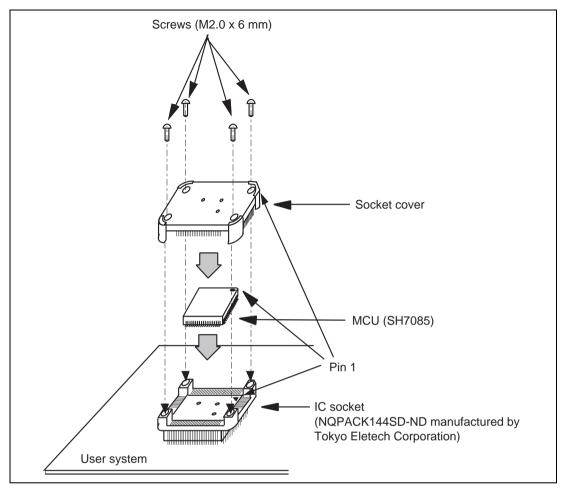
Figure 11 Installing MCU to User System
